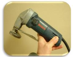
When using welded-wire mesh, renting a metal-cutting shears can help considerably if you are cutting lots of mesh for a big job, such as a very large deck
